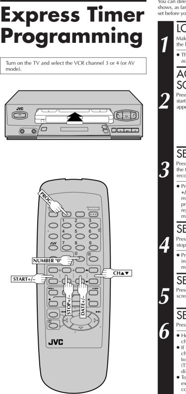
You can directly program the VCR's timer to record up to 8 shows, as far as a year in advance. Remember, the clock must be set before you can program the timer ( $\square pg$ , 6 or 9).
