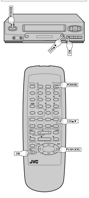
The Plug & Play function simplifies installation by guiding you through the procedures of setting the language, clock and tuner channels — simply follow the on-screen menus that appear when the **POWER** button is first pressed to power on the VCR after you connect the power plug to an AC outlet.
