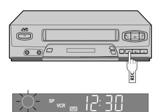
This easy method lets you record from 30 minutes to 6 hours (selectable in 30-min. increments) and shuts the VCR off after recording is finished.
